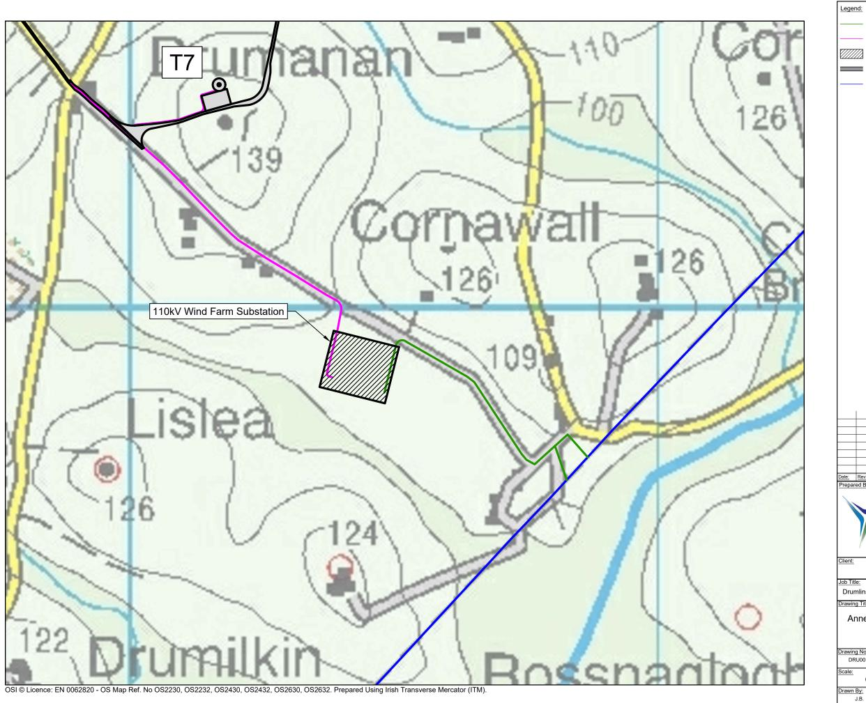
Connection to Existing Overhead 110kV Line Underground Wind Farm Cabling 110kV Wind Farm Substation Wind Farm Access Tracks and Hardstands Existing 110kV Overhead Transmission Line Galetech Energy Services Clondargan, Stradone Co. Cavan, H12 NV06 GALETECH info@galetechenergy.com www.galetechenergy.com Drumlins Park Ltd. Drumlins Park Wind Farm Substation & Grid Connection Annex 2.1 - Alternative Grid Connection Option G3 Drawing No. DRU001SS\_PAG\_ALT-0.03
